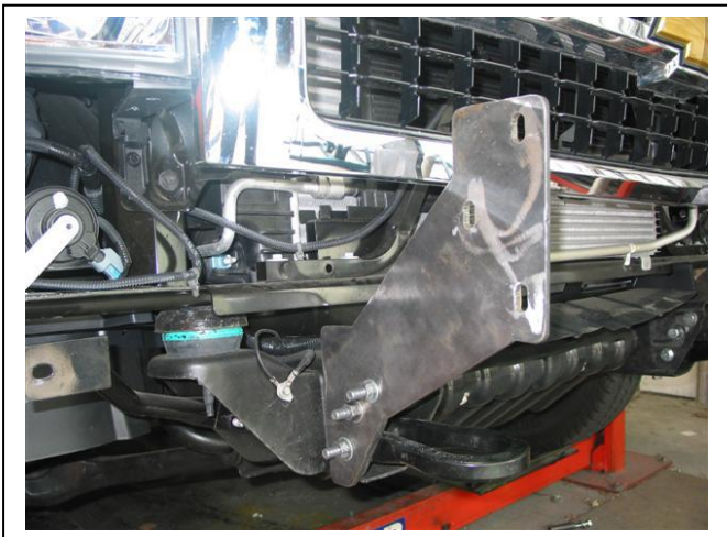
Figure 3: Drivers side steel mounting bracket fitted
