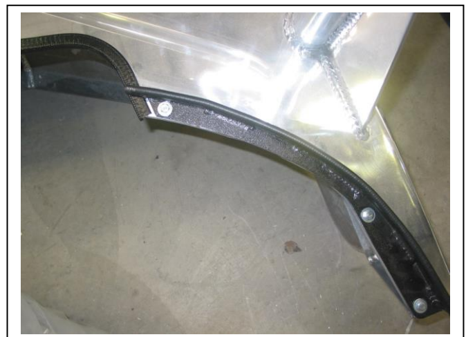
Figure 6: 6mm clip lock trim protrudes past alloy infill and is locked down when bolts are tightened.
