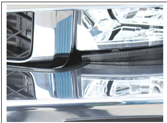
Figure 5: point on bumper alloy infill meets 6mm clip lock trim.
